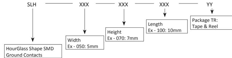
Example: "SLH-050-070-100-TR" for hourglass shape, 5mm in width, 7mm in height and 10mm length in Tape & Reel.
