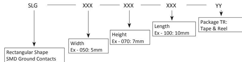
Example: "SLG-050-070-100-TR" for rectangular shape, 5mm in width, 7mm in height and 10mm length in Tape & Reel.
